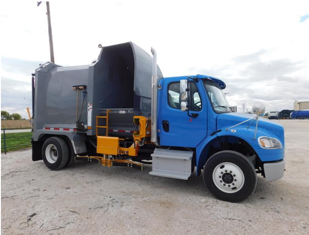
New Way ROTO PAC® 14 CY Automated Side Loader for organics
