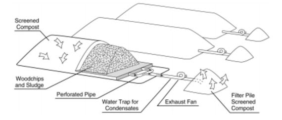
Air is drawn through the composting mass and odorous volatile compounds are removed in a soil biofilter (Willson, 1980).
